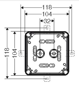
2xM20/25 2x Ø9-17 mm 2x Ø9-17 mm 2xM20/25 2xM20/25 1x Ø9-17 mm
